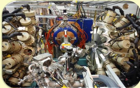
The Gammasphere array and target chamber at ANL.
