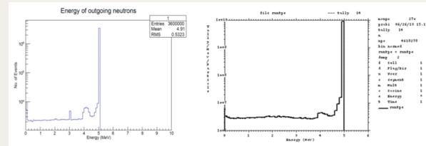
Figure 7: Comparison of neutron scattering in Geant4(left) and MCNP(right)
