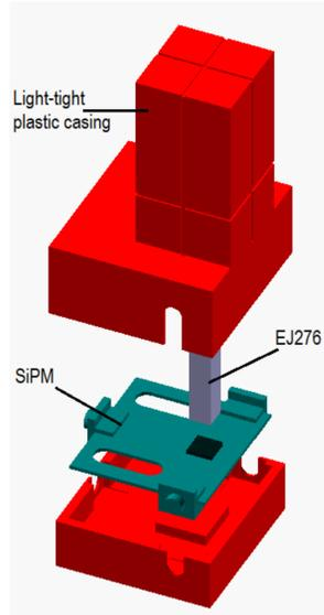
The prototype of the compact neutron spectrometer consists of a 6x6x50 mm<sup>3</sup> EJ-276 plastic scintillator coupled to a silicon photomultiplier (SiPM) in a light tight casing operated at +28.5 V using an external power supply. The reference detector is a 50 x 50 mm<sup>2</sup> cylindrical EJ-301 liquid scintillator coupled to a 12-stage photomultiplier tube operated at a bias of 1000 V.
