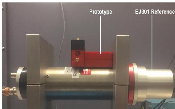
Measurements of a 2.2 GBq americium-beryllium (AmBe) source and 14.1 MeV neutrons from a sealed tube neutron generator (STNG) were made at the n-lab in the Department of Physics at UCT using the prototype and reference detectors.
