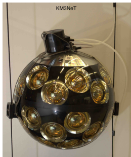
Figure – KM3NeT real DOM vs simulated DOM by the PTM code.
