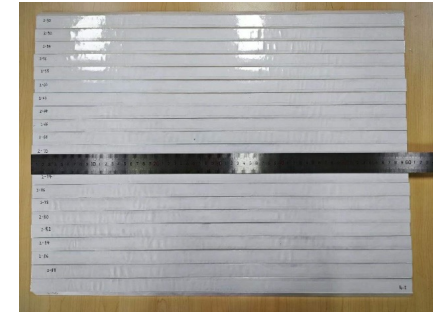
Scintillator machining and wrapping
