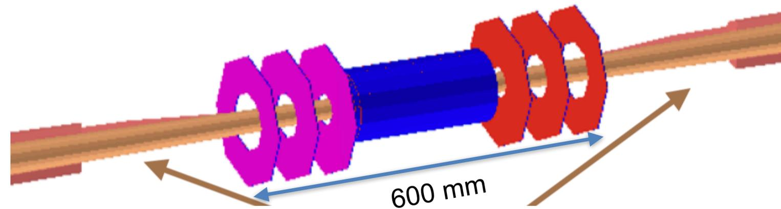
3 double barrel layers + 3 double-layer disks per side
