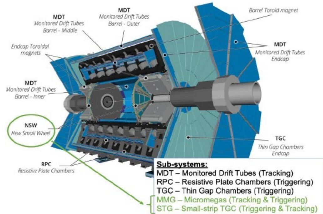
The Atlas Muon Spectrometer
