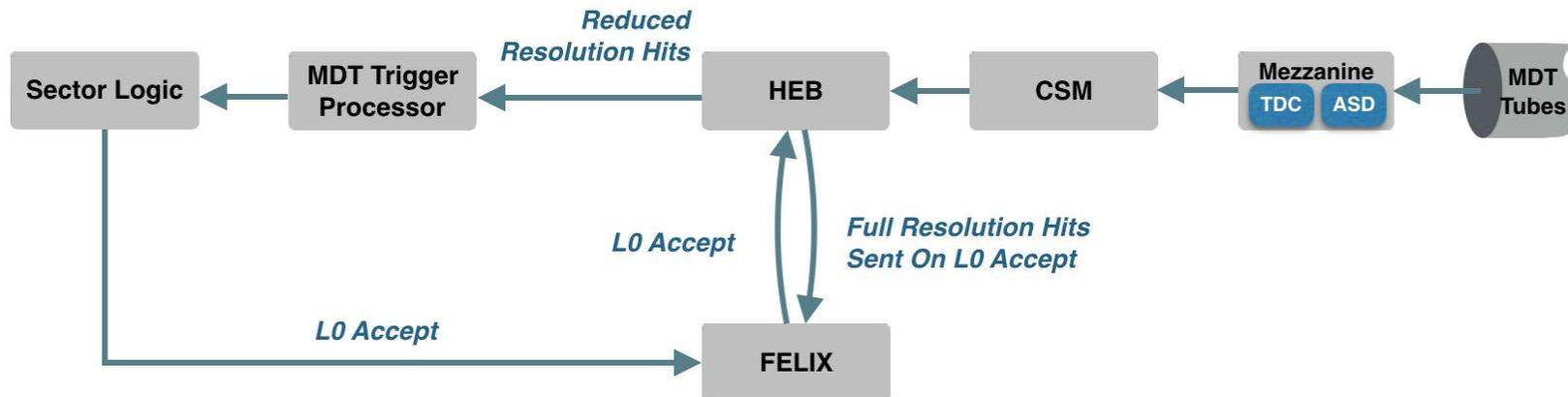
The new architecture for the MDT trigger and readout system in Phase II.
