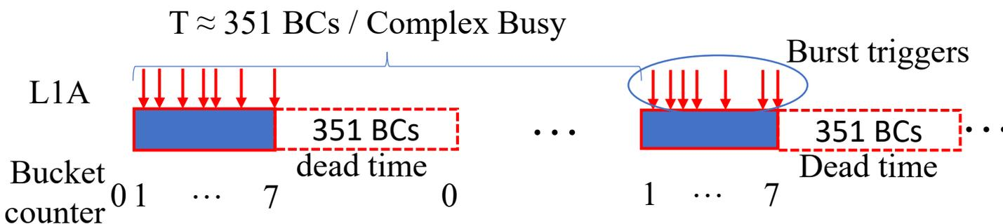
**Burst triggers & complex dead time for the simulation**
