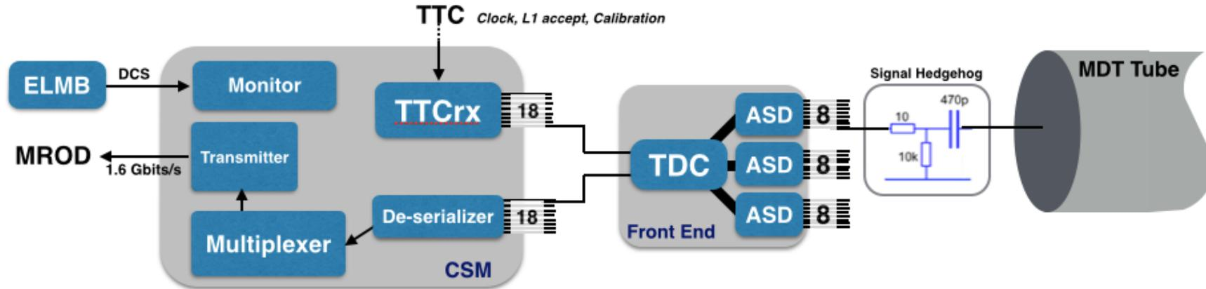
Block diagram of the present MDT trigger and readout system
