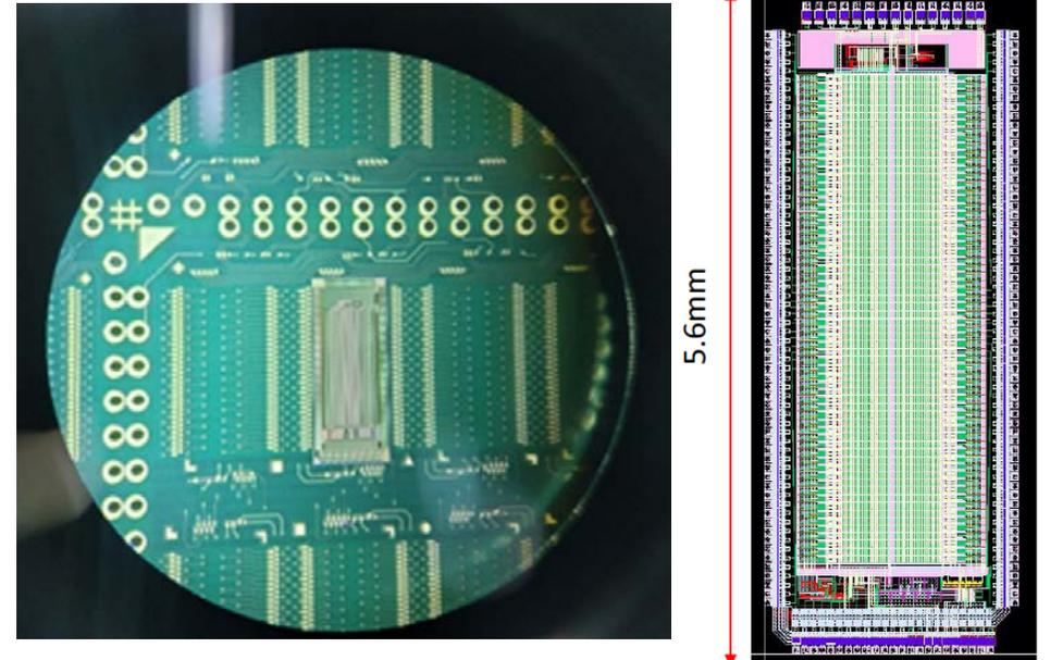
1<sup>st</sup> readout PCB board and the ASIC layout
