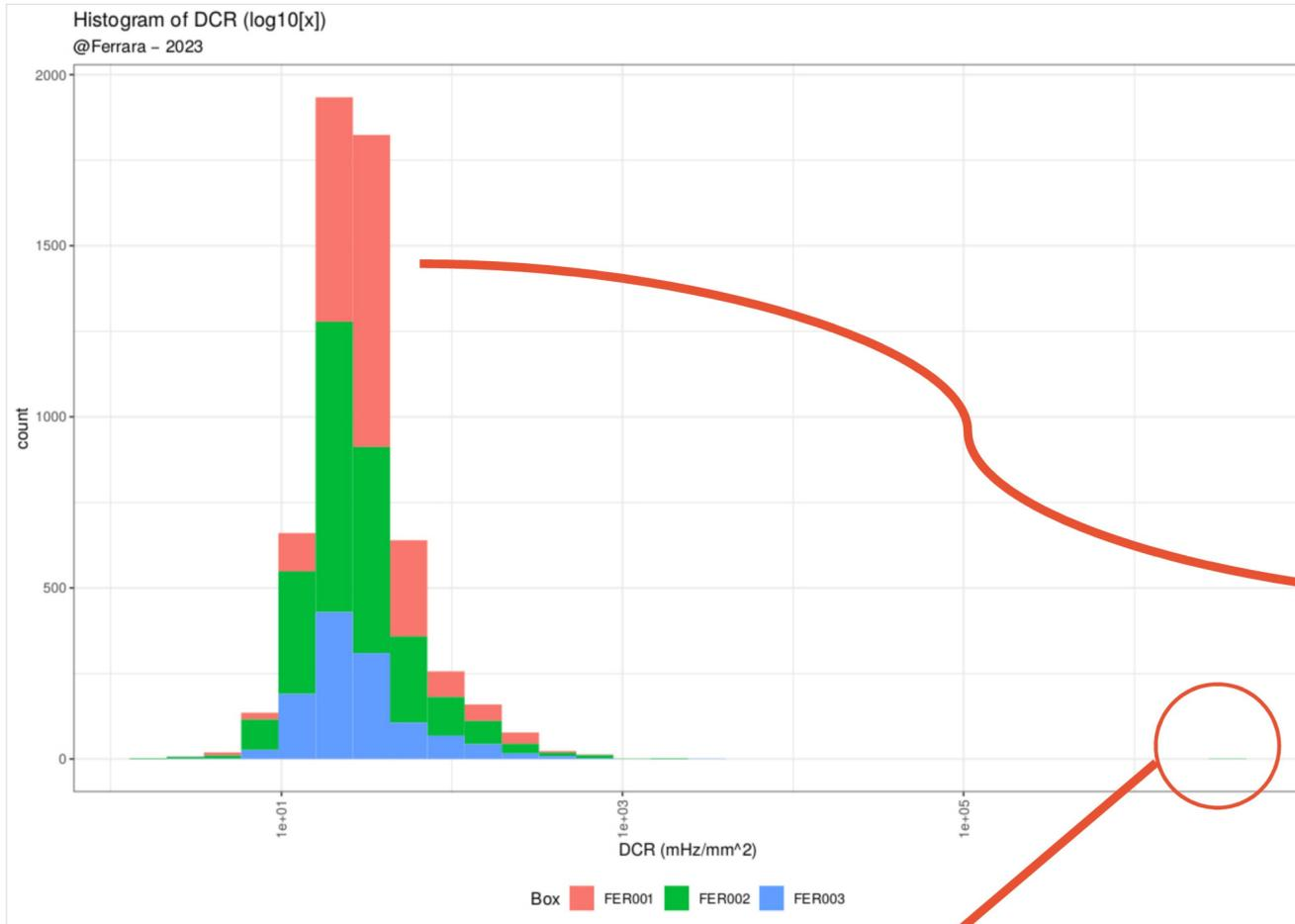
DCR in specs for almost all SiPM (<200mHz/mm<sup>2</sup>)
