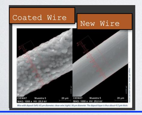
The electron avalanche enable chemical reactions of impurities creating a coating on the wires
