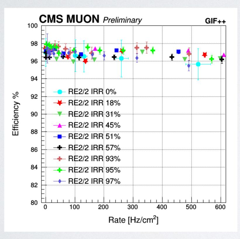
• results obtained during Test Beam with source on (simulating background rates)
