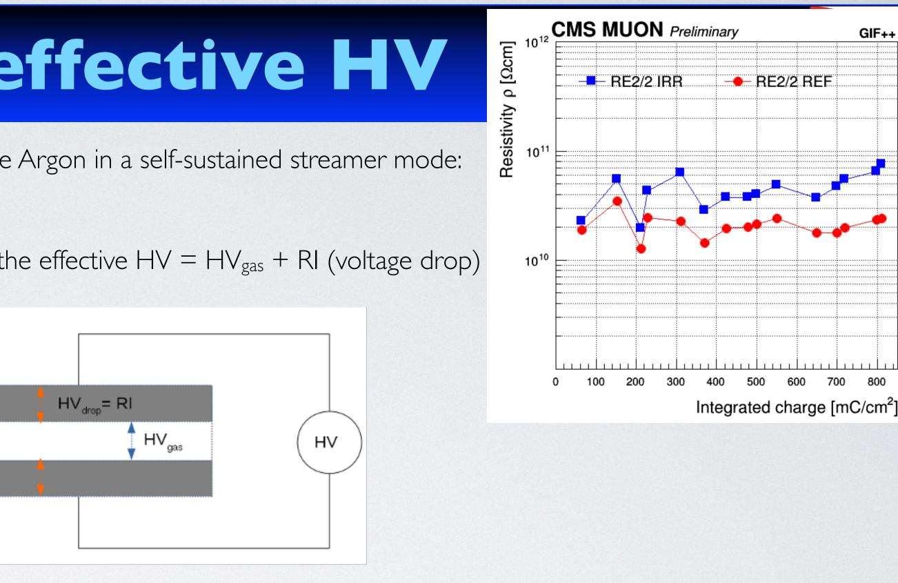
• Performance is measured at the HV working point (WP), defined as the HV at knee + 150 V
