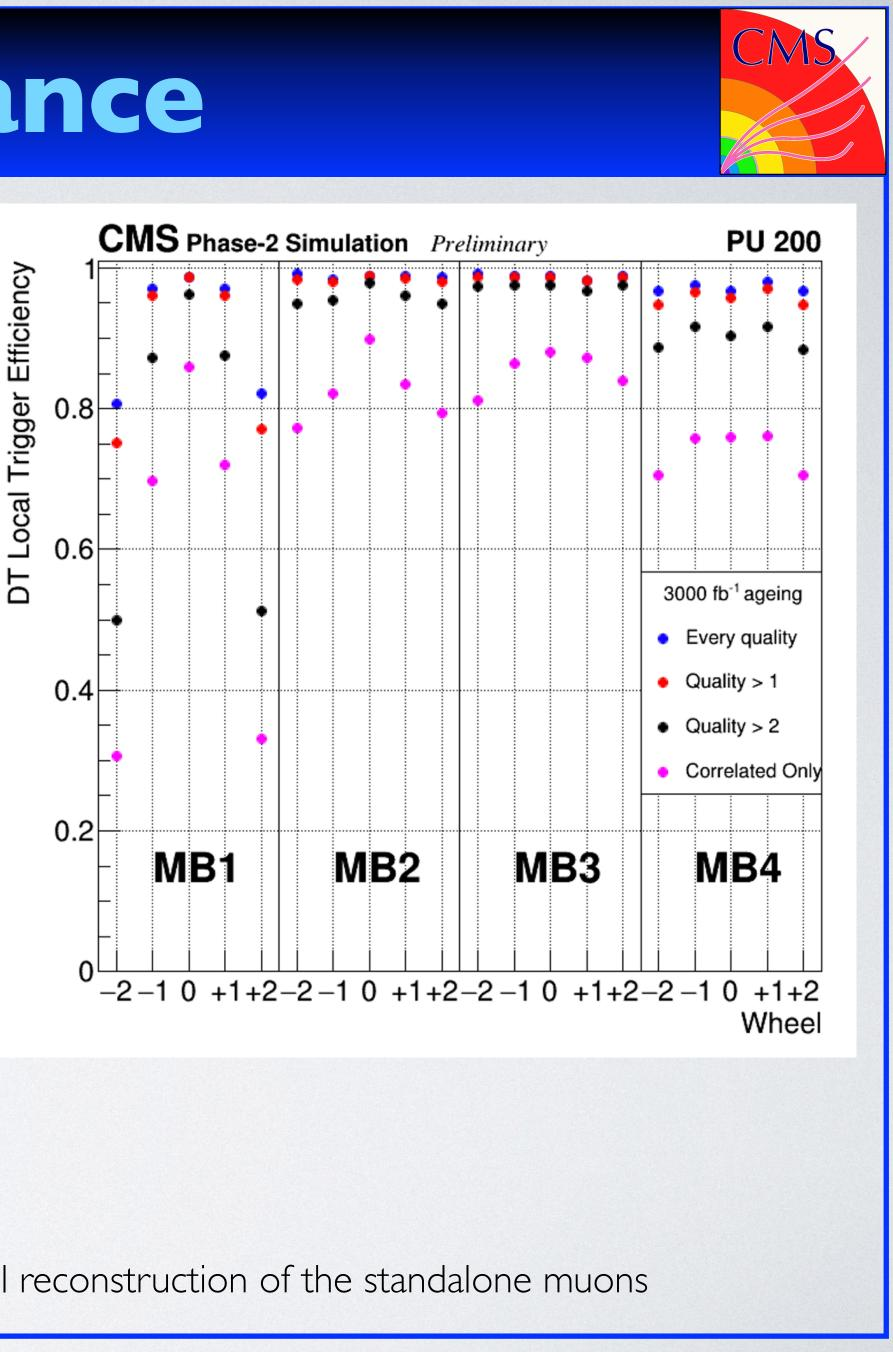
• Minor impact on the overall reconstruction of the standalone muons
