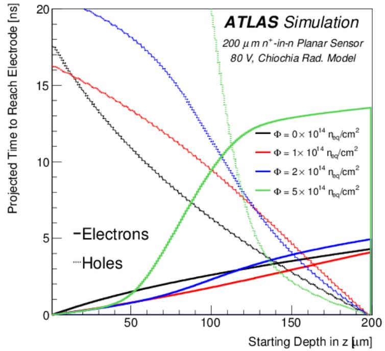
It takes holes much longer on average to arrive at the electrode. Worsens as fluence accumulates
