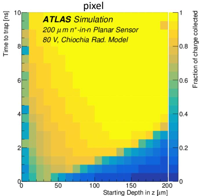
The induced charge includes the contribution from electrons and holes, while the electron time to trap is used for the vertical axis
