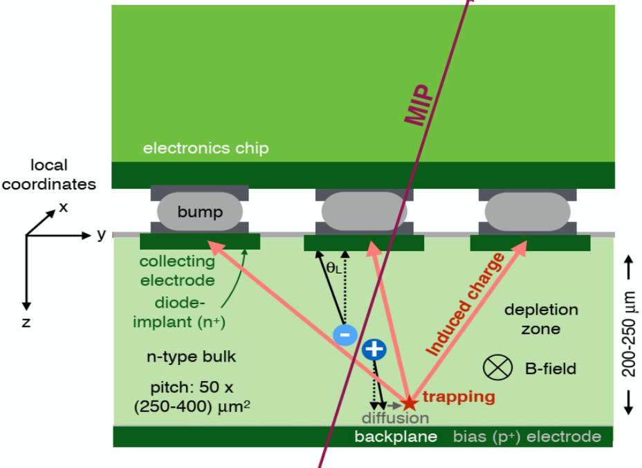
Radiation damage can alter the space-charge density which in turn affects electric field
