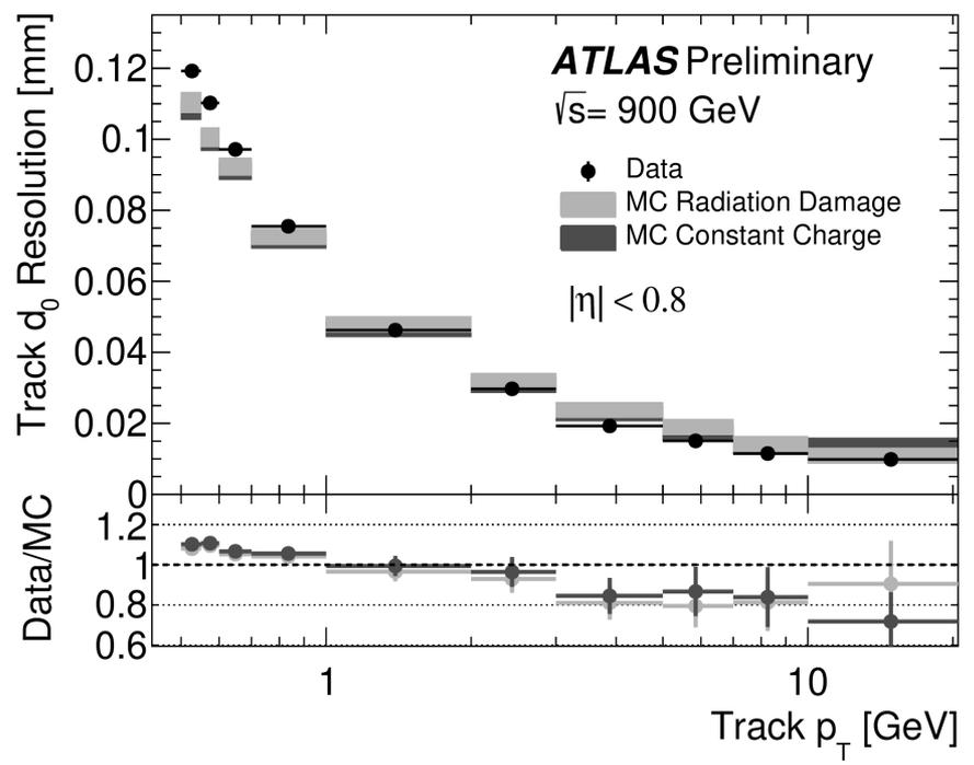
The tracking performance of the ATLAS Pixel Detector is not much affected by radiation damage for the fluence integrated so far. This is shown by the similarity of the results using radiation damage and the constant charge MC samples
