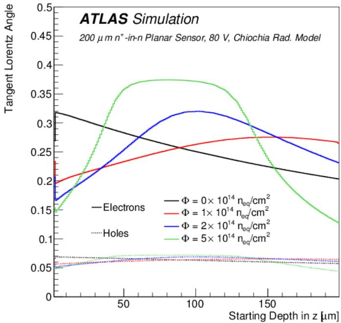
As the mobility increases with decreasing electric field strength, the Lorentz angle is largest near the center of the irradiated sensors
