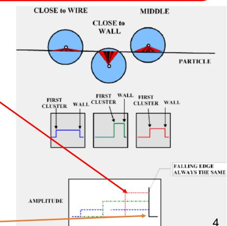
Straws operate in the proportional mode, so the total charge *q* of the iduced signal is proportional to the ionization energy loses dE/dx and may serve PID
