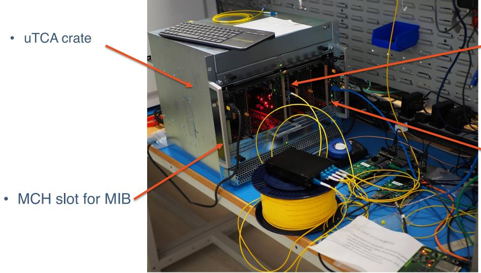
AFC into an AMC slot •
