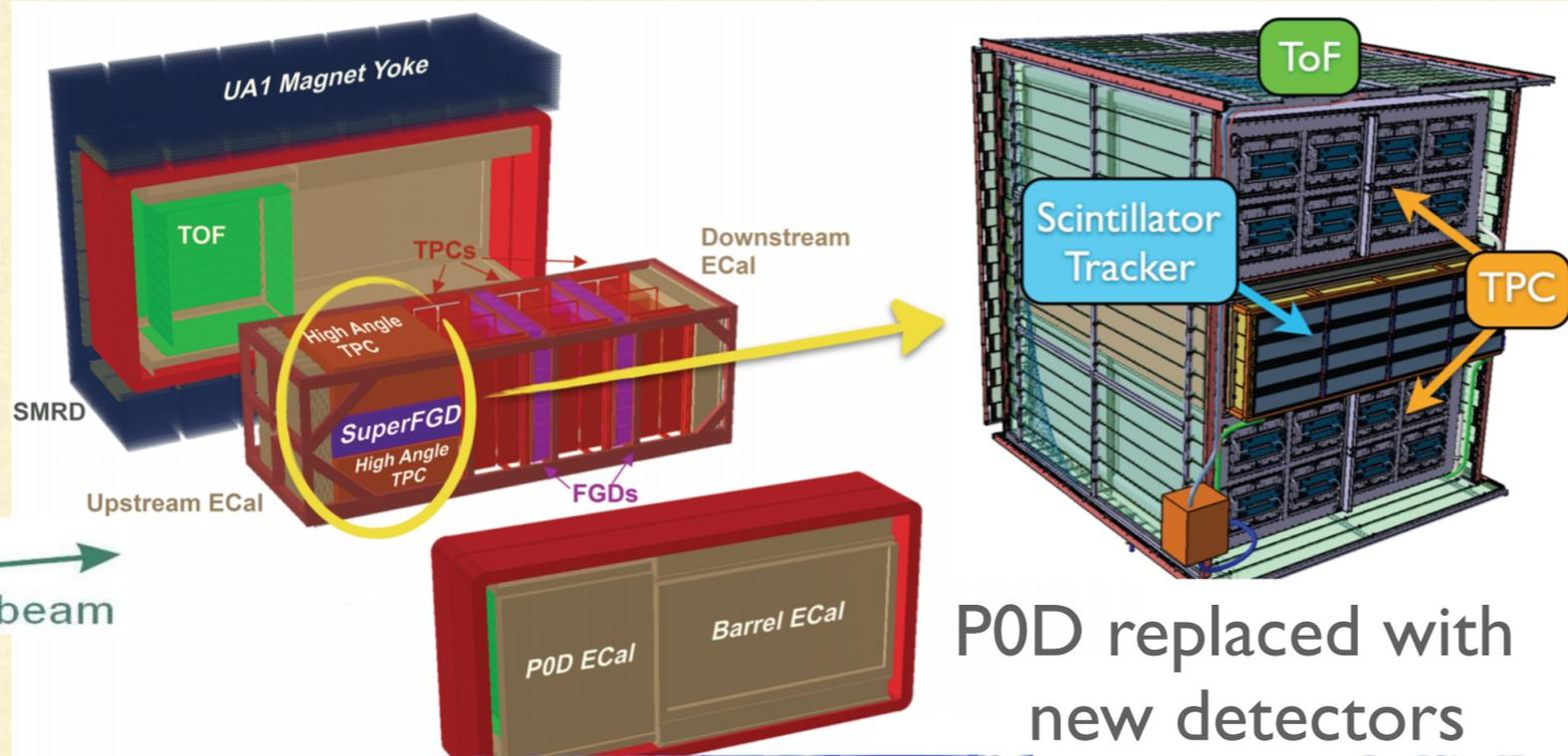
P0D replaced with new detectors
