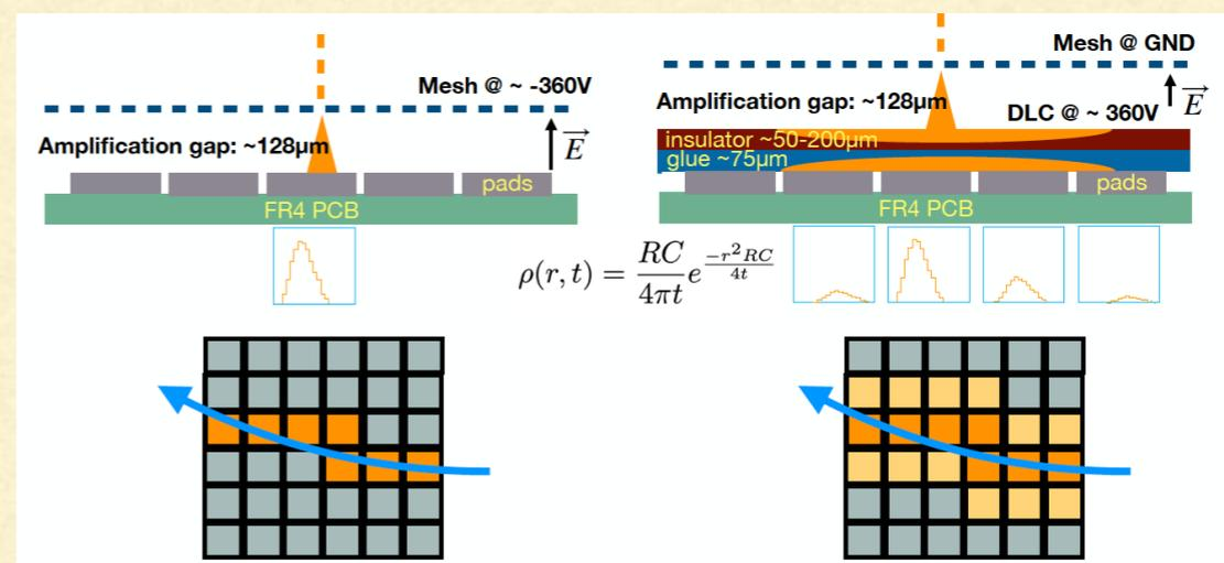
Encapsulated Resistive Anode Micromegas (ERAM) with grounded mesh, anode at a positive amplification voltage
