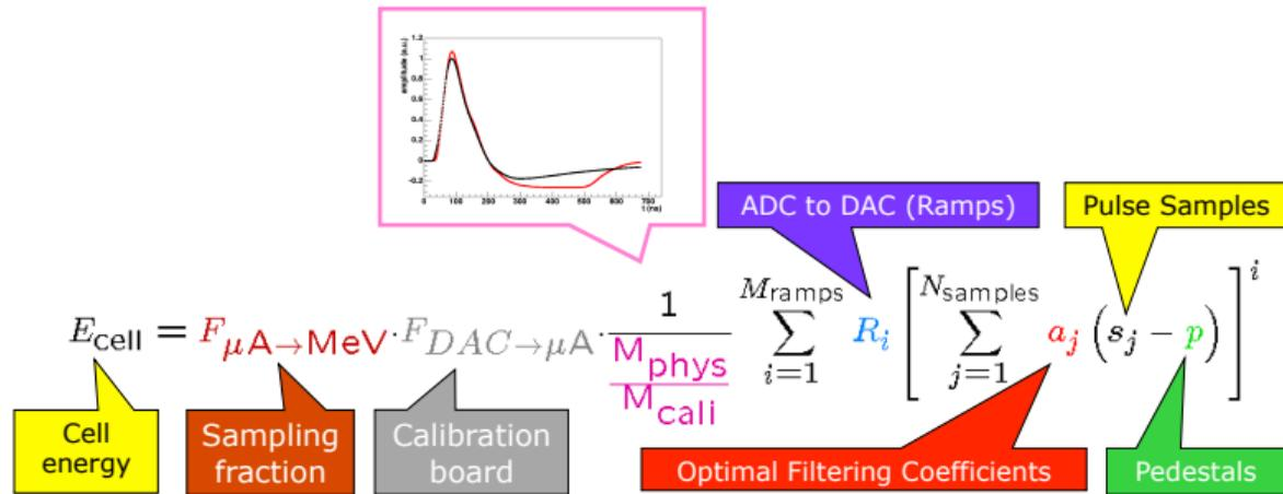
The above formula describes the LAr electronic calibration chain (from the signal ADC samples to the raw energy in the cell). Note that this version of the formula uses the general  $M_{\text{ramps}}$ -order polynomial fit of the ramps. We use a linear fit as the electronics are very linear, and we only want to apply a linear gain in the DSP in order to be able to undo it offline, and apply a more refined calibration. In this case, the formula is simply:
