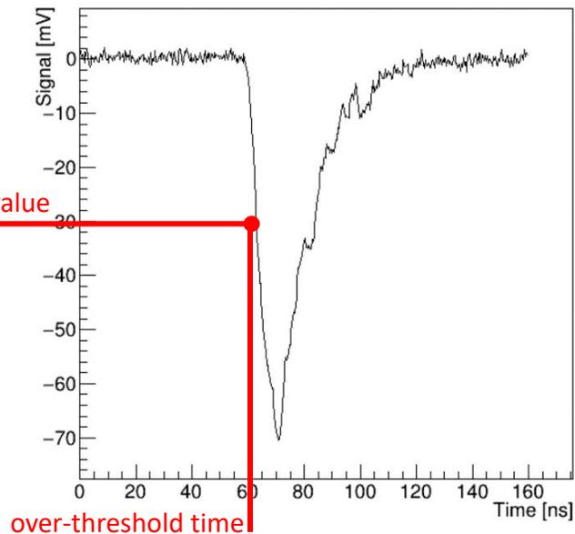
leading edge timing to determine over-threshold time
