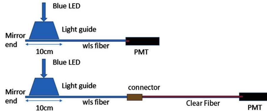
10-10 WLS fibers coupling to clear fibers (length 1 m ) with **Fujikura** connector.
