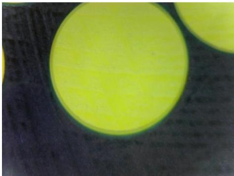
fiber end after polished under microscope
