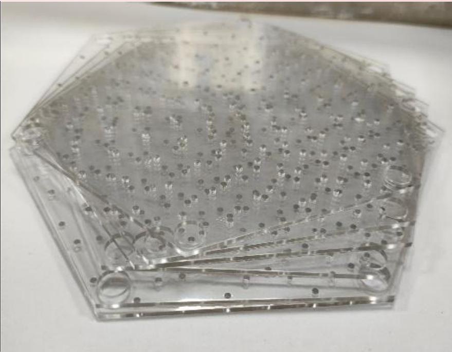
plastic scintillator, produced with injection mold
