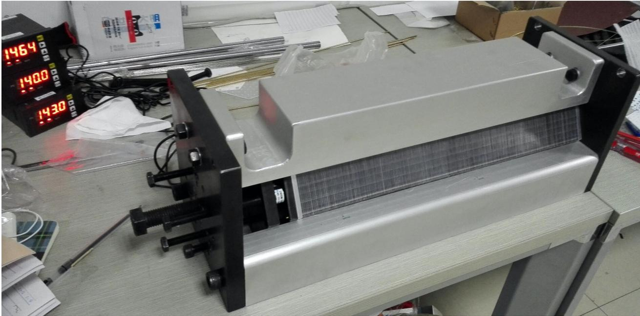
Scintillator tiles and leads are cross stacked in the mould, keeping pressure stable on ECal for hours.
