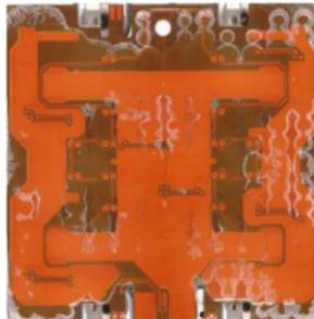
Glue pattern after using the final prototype stencil: continuous glue layer
