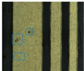
Chemical contaminations and scratch on a pad.
