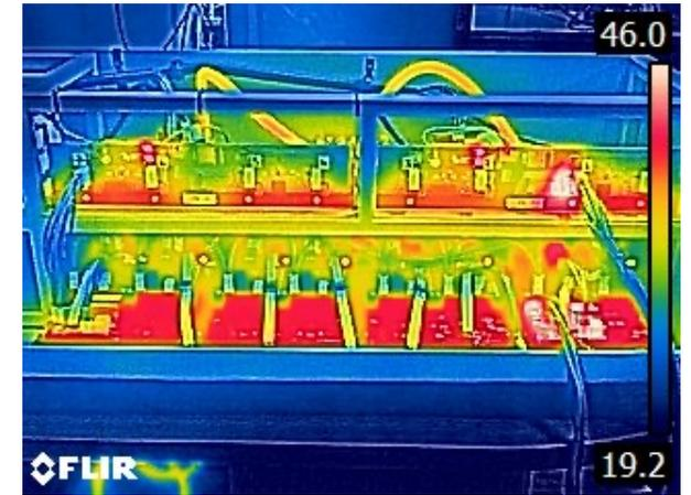
Fig. V8.4.2 Brick undergoing burn-in.
