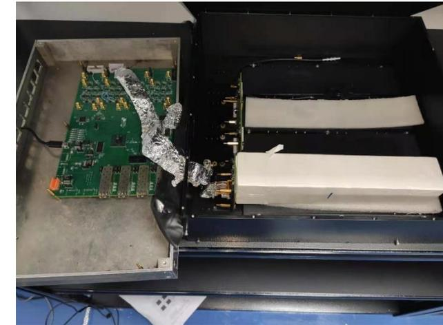
Schematic diagram and photo of the cosmic ray test setup
