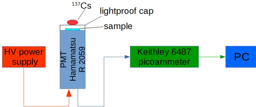
The block diagrams of the test setup
