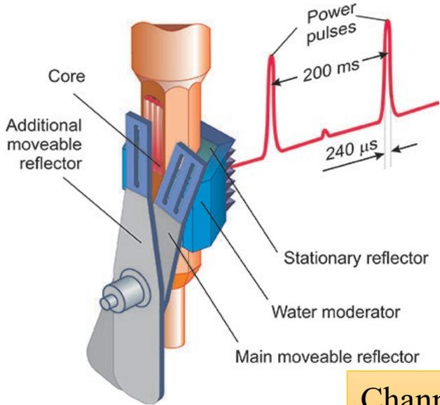
IBR-2 at Frank Laboratory of Neutron Physics, JINR is a pulsed fast reactor of periodic operation. Its main difference from other reactors consists in mechanical reactivity modulation by a movable reflector.
