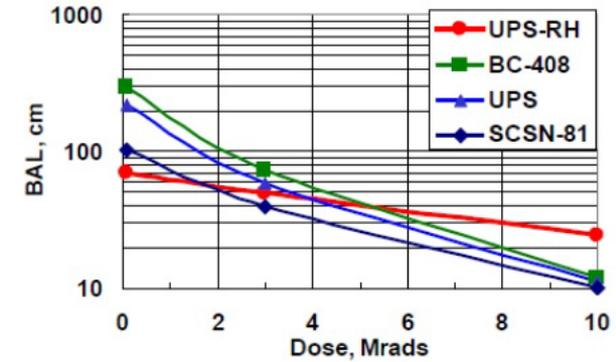
After irradiation the light output loss of the blue scintillator is much higher
