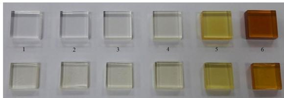
The loss of transparency of the UPS-923A scintillator is much higher in the region of its own fluorescence compared to the green scintillator
