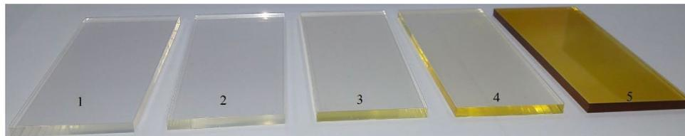
Samples of UPS-923A and green scintillators were irradiated in wide range of neutron fluence. All samples are produced by ISMA, Kharkov.
