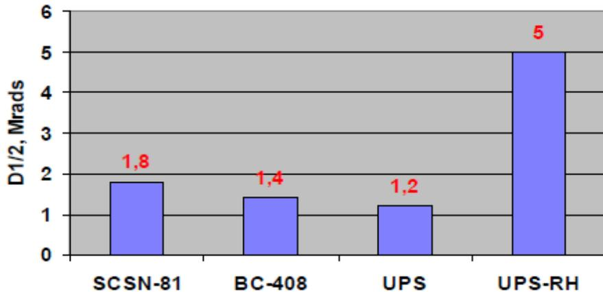
Dose when the light yield drops two times for different scintillators
