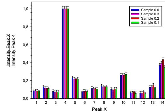
From Raman spectra we did not find structural changes or damage occurred during the neutron irradiation up to  $1.8 \cdot 10^{14} \text{ n/cm}^2$ !
