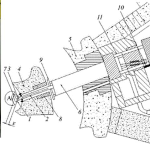
During a running cycle fluence is  $10^{18}$  n/cm<sup>2</sup> on the I-beam end and  $10^{16}$  n/cm<sup>2</sup> and  $10^{11}$  n/cm<sup>2</sup> on the pipe beginning and end respectively
