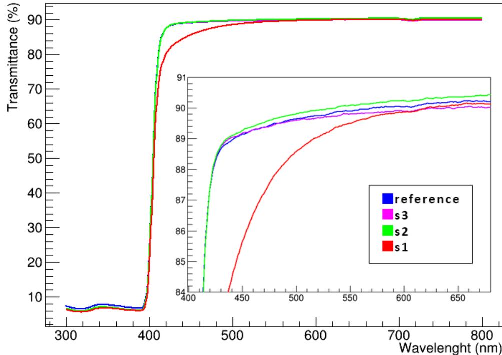
Fluens  $\sim 10^{14}$  n/cm<sup>2</sup> resulted in a few percents light transmission loss in the range of 400-550 nm
