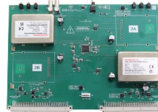
prototype HV supply board
