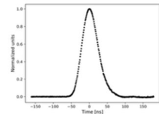
Pulse shape in HG from 2022 test-beam data
