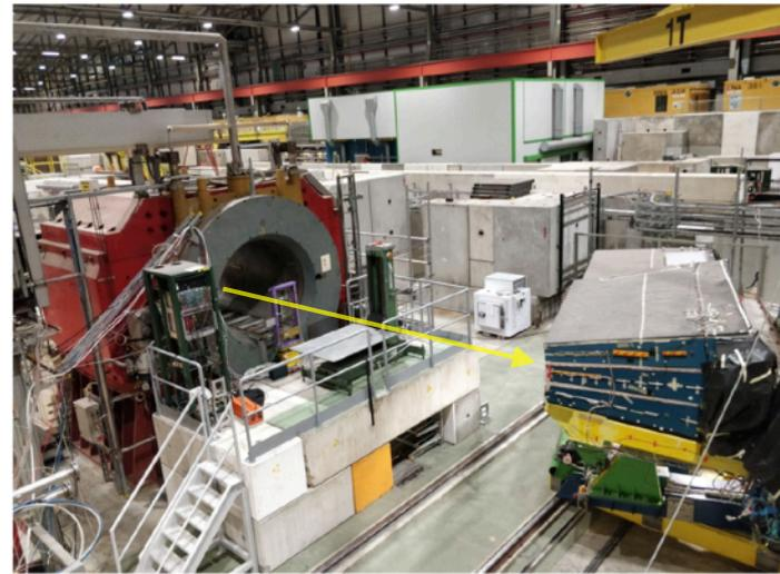
TileCal setup in the SPS-H8 beam-line.
