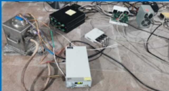
JINR Precision Laser Inclinator installed in Garmy Geophysical Observatory (GGO)
