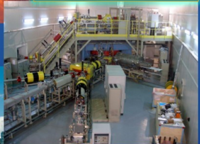
DC-60 is a heavy ion accelerator (isochronous cyclotron), built in 2006 in Astana. The cyclotron project was developed at JINR
