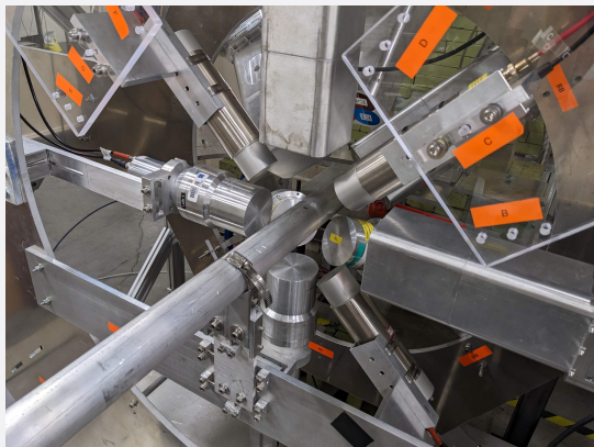
\gamma -ray detectors around the target position.
