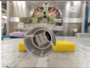
Target pipe, target holder inside the pipe and the target.
