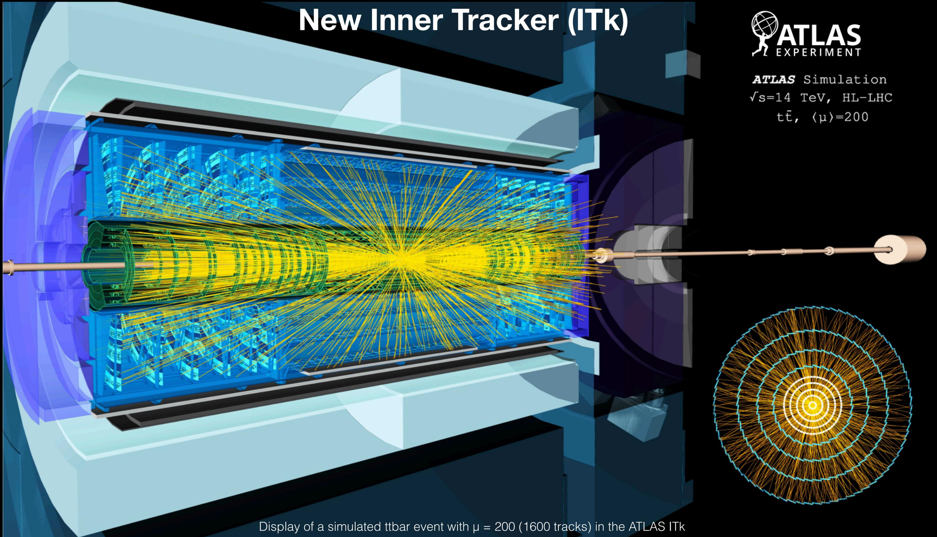
Display of a simulated  $t\bar{t}$  event with  $\mu = 200$  (1600 tracks) in the ATLAS ITk
