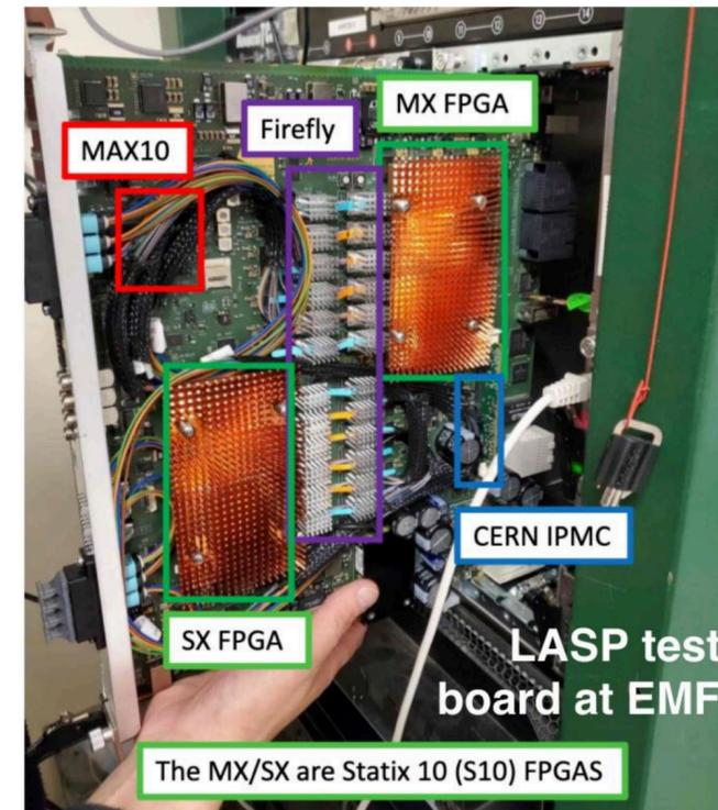
LAr Signal Processing test board
