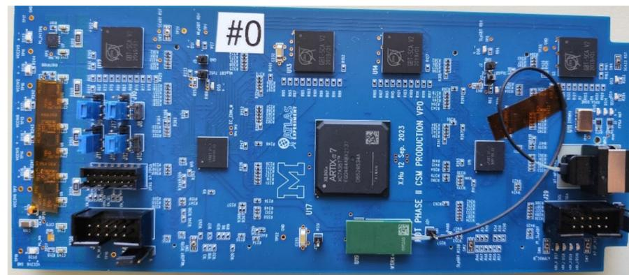
Muon Chamber Service Module board
