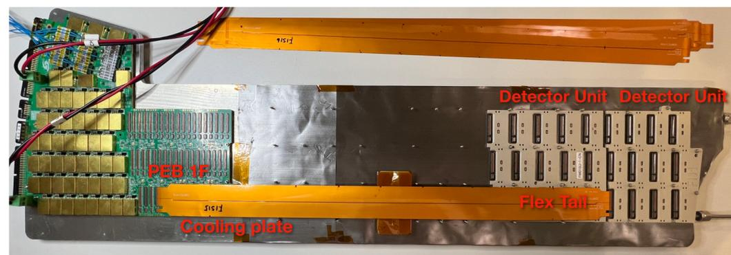
HGTD peripheral elx board prototype
