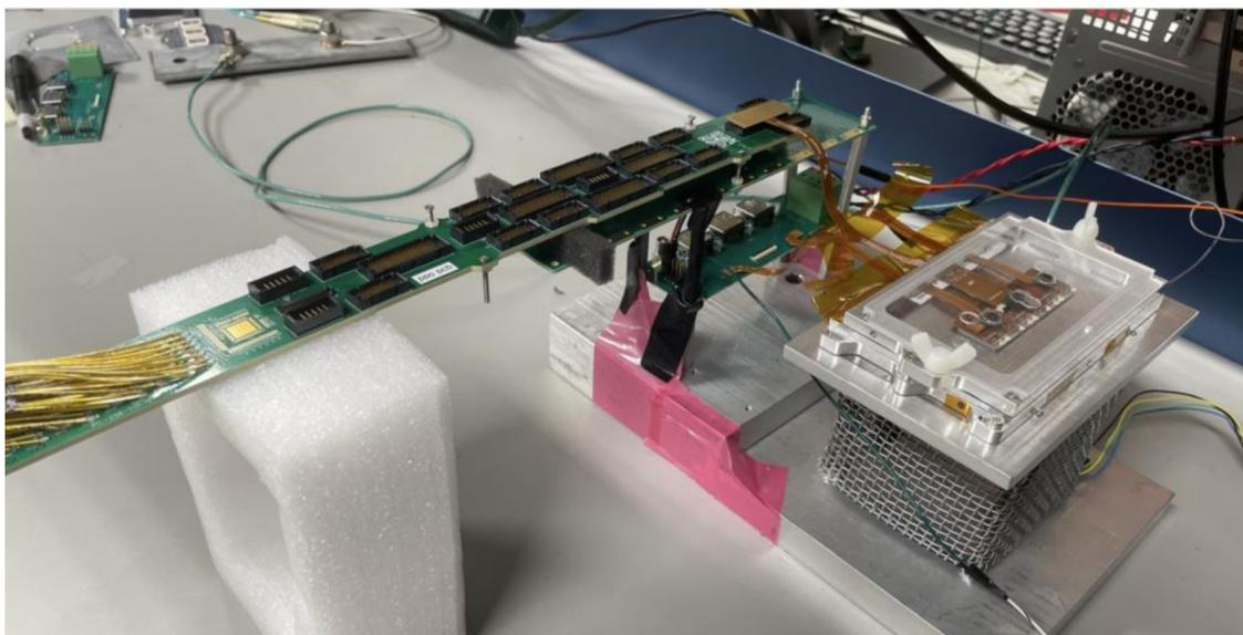
ITk Pixel full data transmission test
