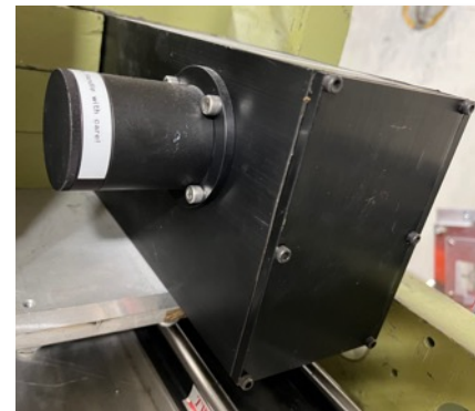
Alignment – BGO CCD gamma camera & lead plugs:
