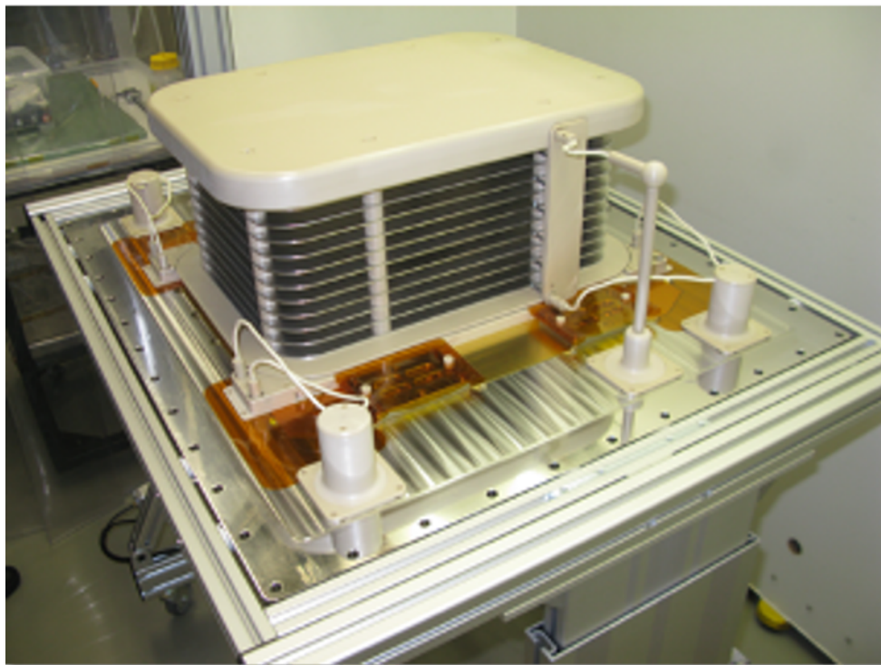
Fully assembled TPC structure with 33 \times 20 \times 19.6 \text{ cm}^3 fiducial volume
