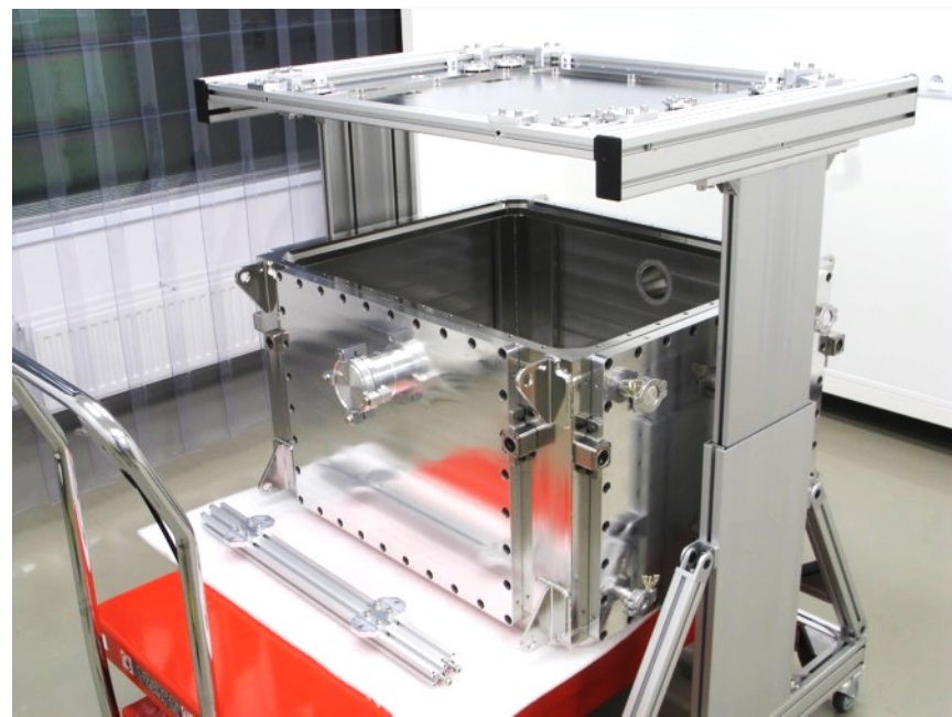
Vacuum vessel (250 \text{dm}^3 ) with removable endcaps & side walls
