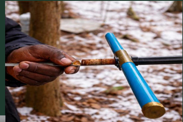
Increment borer sampling at Yamakiya, Fukushima
