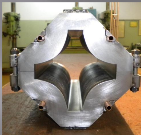
yoke of quadrupole lens after final treatment
