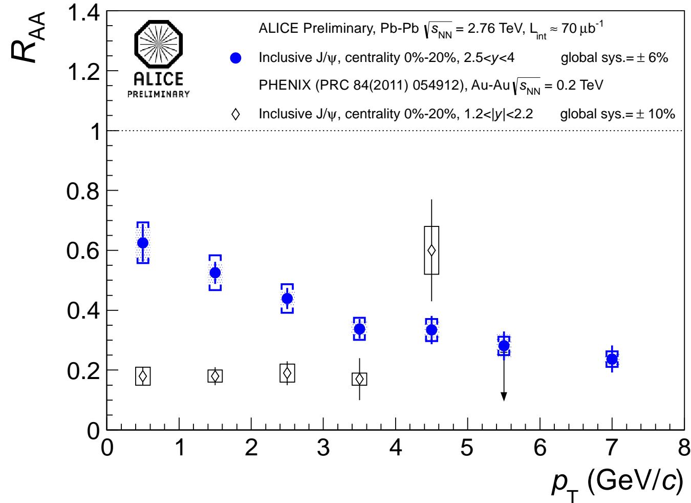
Different production patterns at the LHC compared to RHIC energy further support for (re)generation mechanisms
