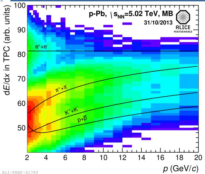
This is done in the relativistic rise regime of the Bethe-Bloch curve, where the <d*E*/d*x*> separation between particles with different masses is nearly constant.
