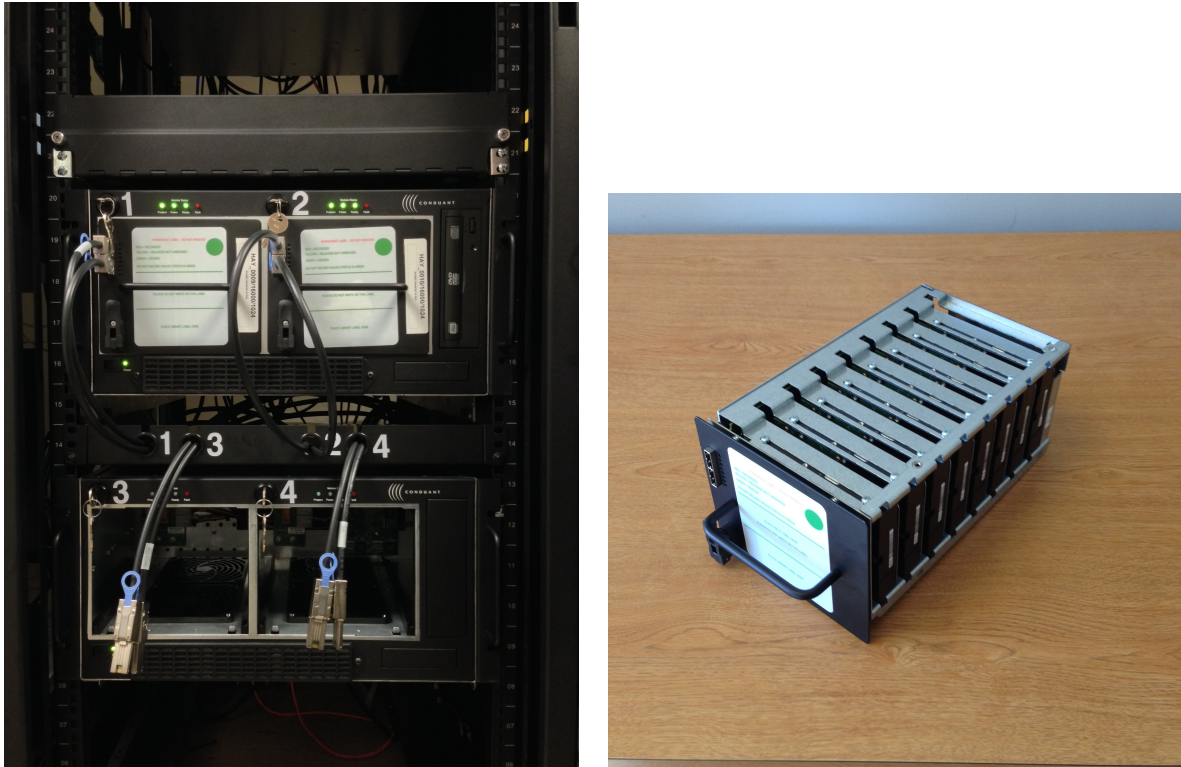
Figure 12. The left panel shows a photo of a Mark6 data recorder, and the right panel a photo of a disk pack, or “8-pack” which might currently carry eight 6-terabyte commercial hard disk drives for 48 TB of storage.
