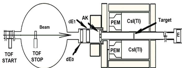
**Figure 1.** The scheme of the experiment for measurement of reaction cross sections using  $4\pi$ -scintillation  $\gamma$ -spectrometer.
