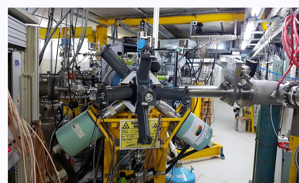
Fig.10. Complete array of electrometer connected to g-line.
