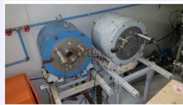
Fig.1. SK magnetic lens (solenoid) previously used at Orsay
