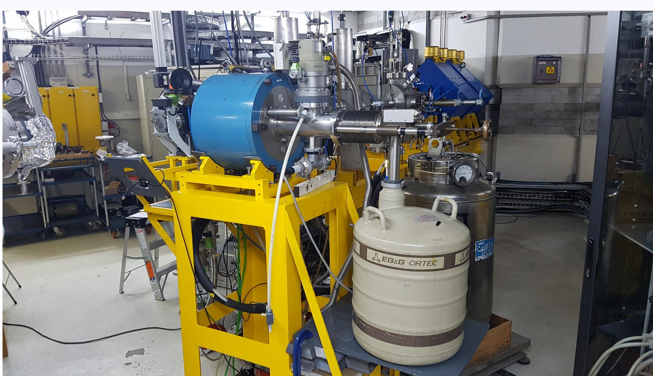
Fig.3. Connection of electron spectrometer to beam line
