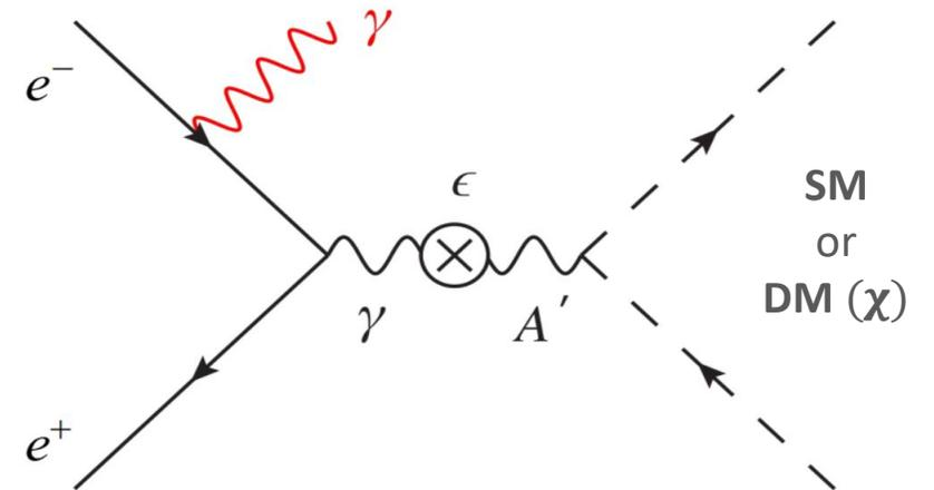
First exploring the invisible decay:  $e^+e^- \rightarrow \gamma_{ISR} A' \rightarrow \gamma_{ISR} \chi \bar{\chi}$
