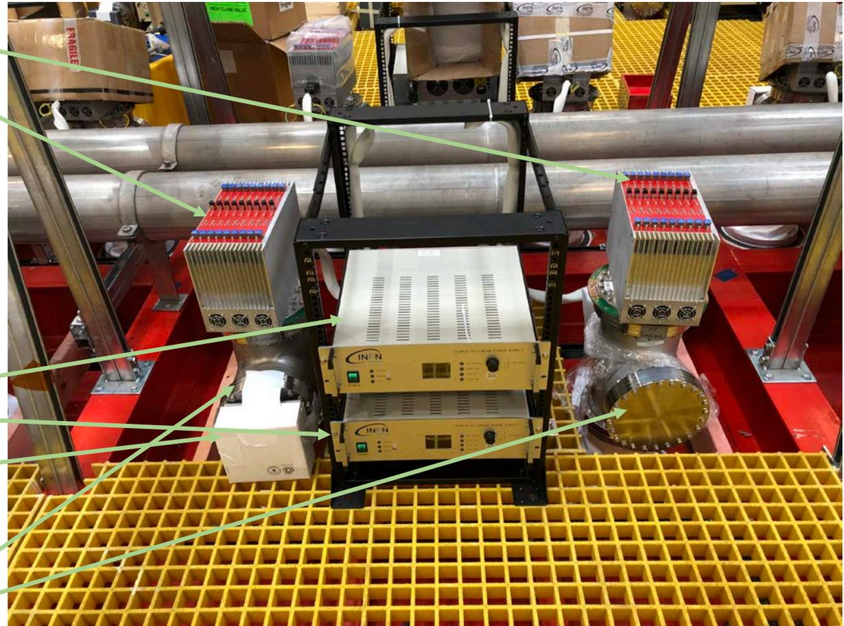
HV and signal feedthroughs for the PMT's are on the back side of the crosses
