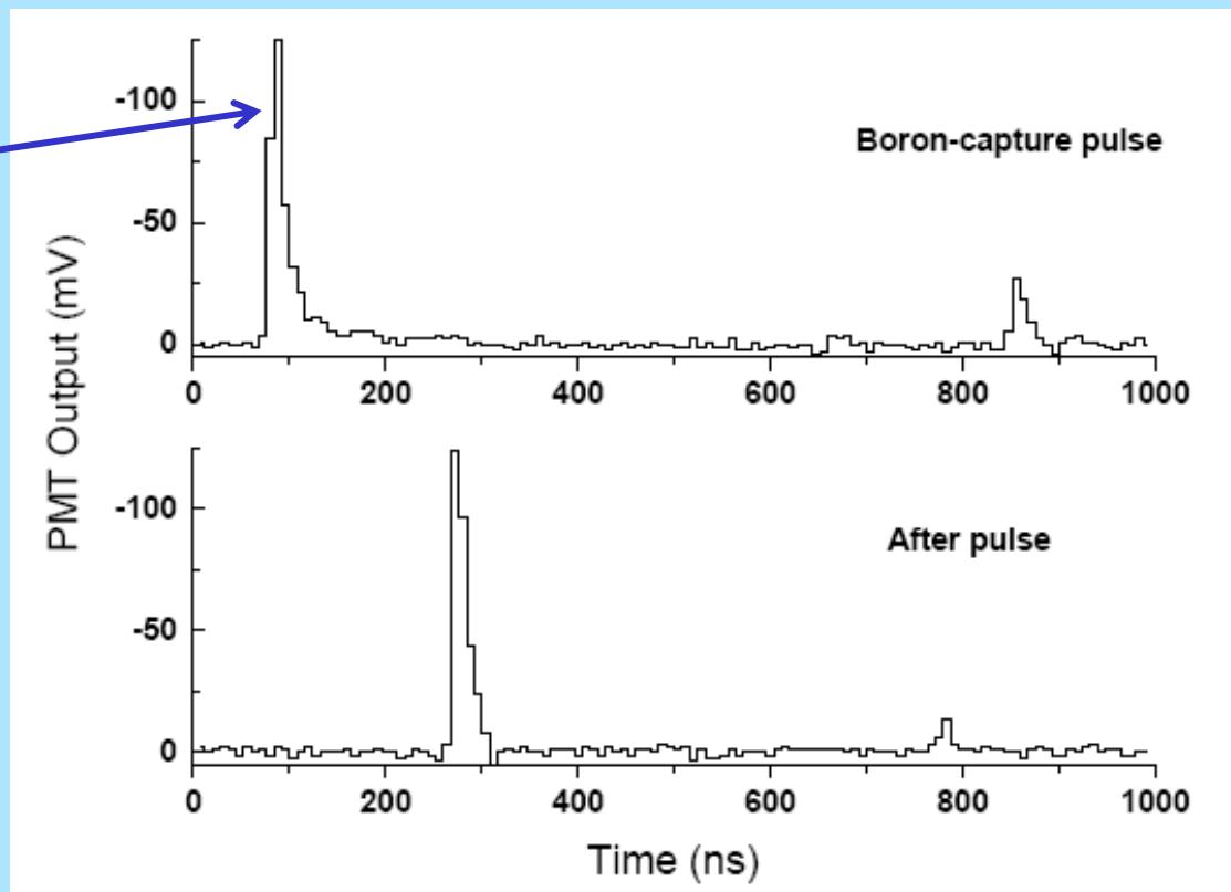
Small pulses require small scintillators !!      Detector must be highly modular!!!
