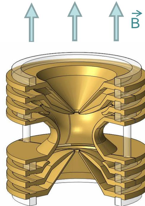
The free cyclotron frequency is inverse proportional to the mass of the ion!
