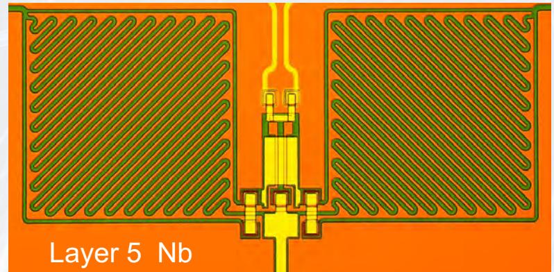
superconducting switch and bridges
