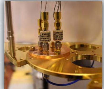
**dc wiring and SQUID array installation**
