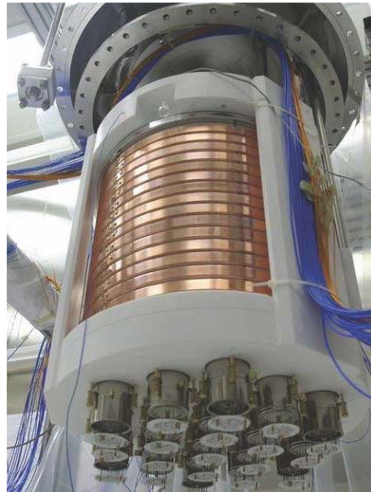
DarkSide-50 at LNGS Active Target: 50kg
