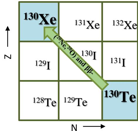
DCE reaction  $^{130}\text{Te}(\beta^- \text{Ne}, \text{O})^{130}\text{Xe}$
