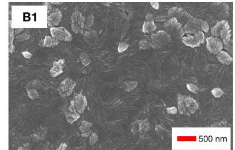
FESEM image of Te target on  $5 \mu\text{m}$  HOPG
