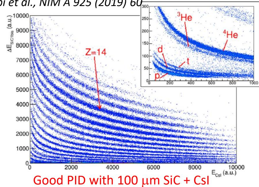
Good PID with 100  $\mu\text{m}$  SiC + CsI
